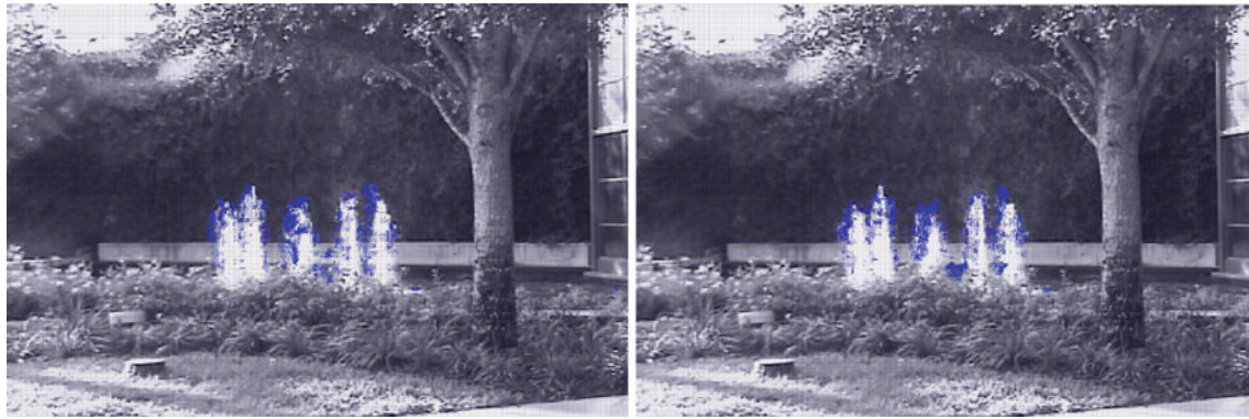
Fig. 1 Sample images from the fountain sequence showing the flow vectors super-imposed on the original image. Sequences such as these, contain dynamic and periodic motions, causing challenges for the traditional approaches
