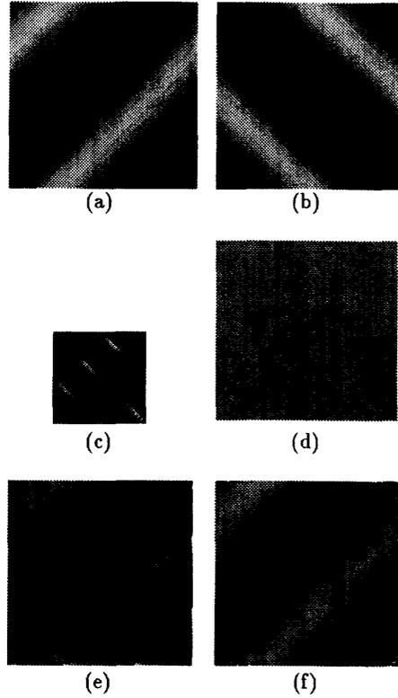
Figure 2: (a) Ideal albedo, (b) ideal altitude, (c) one of the 9 low resolution simulated camera images, (d) Initialization, (e) and (f) reconstructed albedo after the 1st and the 4th iteration.
