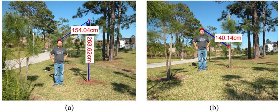
Figure 6: Measurements which might be difficult in practice: (a) The height of the pine is around 264cm, and the distance from the head of the standing people to the top of the pine is 154cm. (b)The distance from the head of the standing people to the top of the stick is around 140cm.
