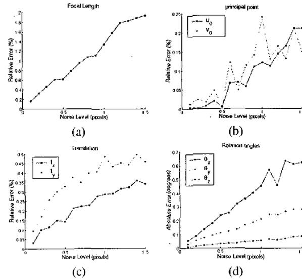
Fig. 2. Performance vs noise (in pixels) using  $u_0 - v_0 - f$  search space, averaged over 100 independent trials: (a), (b) and (c) relative error for  $f$ , principal point and translation, (d) absolute errors in and rotation angles.
