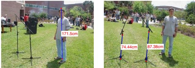
**Fig. 3.** Standing person has known height. Heights of the two microphone stands are computed using our approach.
