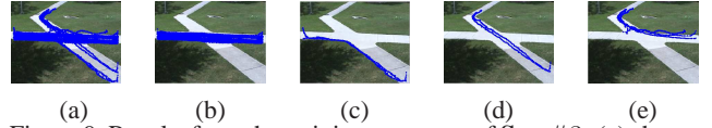
Figure 9. Results from the training sequence of Seq #3: (a) shows all the trajectories used in the training set. (b)-(e) are the 4 paths clustered from the input data.
