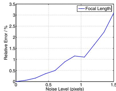
**Figure 2. Performance of the self-calibration method VS. noise level in pixels.**
