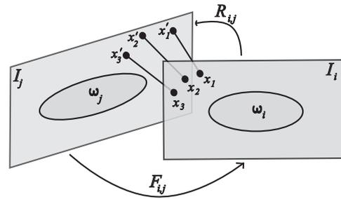
**Figure 1. Illustration of two views from a camera: Two consecutive images from a camera contain an overlapping area. This overlapping area can be used to obtain the fundamental matrix  $\mathbf{F}_{i,j}$ , which relates a point in image  $I_j$  to a line in image  $I_i$ . As the internal parameters change at each view, the absolute conic  $\omega$  also changes.**
