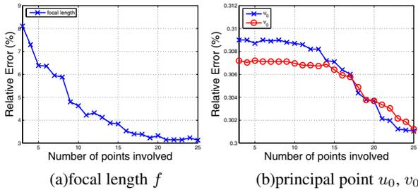
**Figure 3.** Relative errors as functions of number of shadow points
