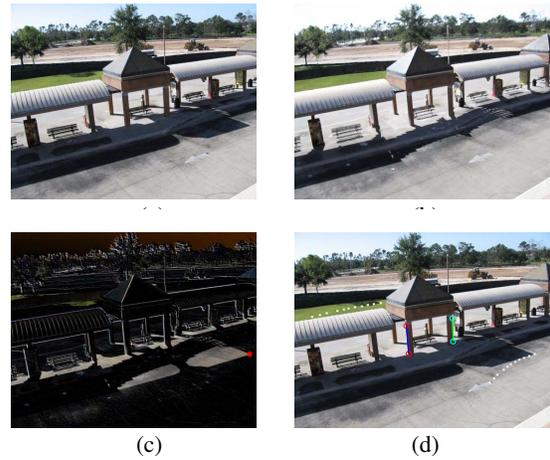
**Figure 5.** (a)A frame of real data (b)Computed background. (c)Shadow point tracking from background subtraction. (d)Shadow trajectories for a roof corner and the top of a tree
