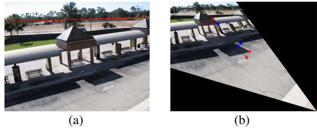
**Figure 6.** Image-based Metrology (a)Computed horizon line  $\mathbf{l}_\infty$ . (b)Two 3D points and their corresponding shadows in different time after affine transformation
