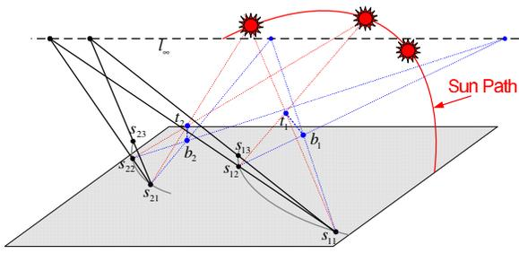
**Figure 1.** The 3D points  $t_i$  cast shadows at different time  $j$  at positions  $s_{ij}$
