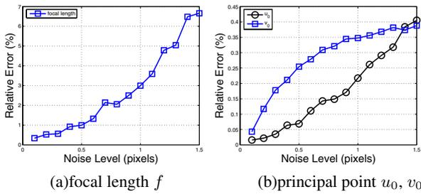
**Figure 2.** Relative errors over different noise levels
